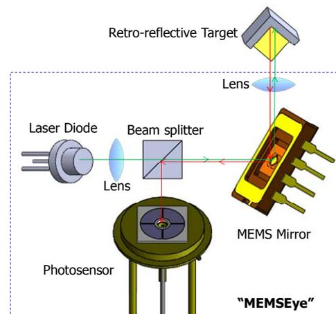
Figure 1. Schematic optical setup for laser-based 3D tracking using a scanning mirror.
