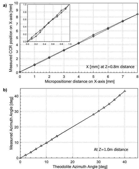
Figure 7. Results from MEMSEye system test for precision using Theodolite. (a) Measurement of precision of change in X-axis position. (b) Measurement results of change in azimuth angle, orthogonal to MEMSEye system.
