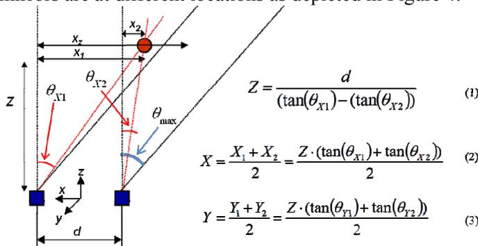
Figure 4. Geometrical setup for two tracking sub-systems which are placed in parallel at a known distance  $d$ , and both track an object simultaneously, thereby obtaining independent azimuth information.
