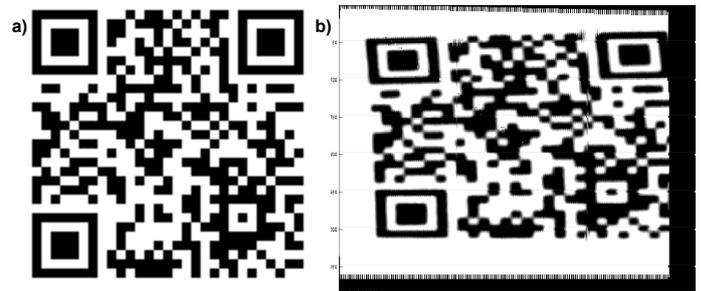
Figure 5. (a) Image of a 2D barcode used for scan tests, (b) result of the MEMSEye scan of the 2D barcode processed and mapped to a  $380 \times 380$  pixel image.
