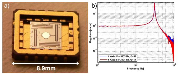
Figure 3. Gimbal-less dual-axis 4-quadrant devices used in this work: (a) typical device which reaches mechanical tilt from -6° to +6° on both axes. Device has a 1mm diameter mirror. (b) Small-signal characteristics of such a high-speed device
