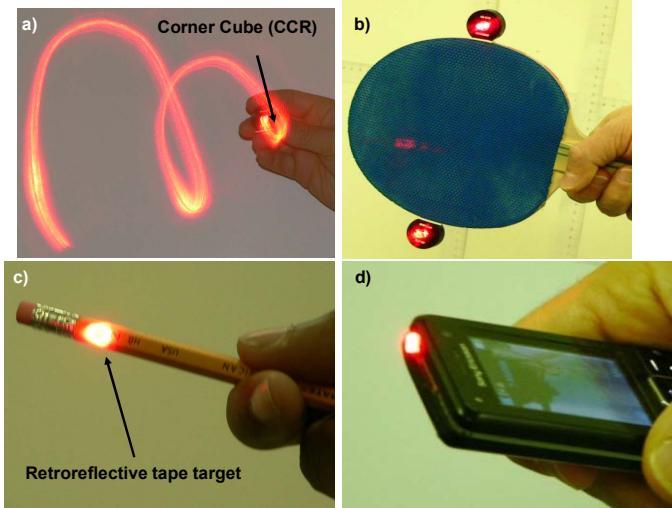
Figure 6. Examples of objects being tracked (targets are bright because the tracking system is actively pointing the laser beam onto them): (a) moving corner-cube retro-reflector, (b) a paddle-marked with two CCRs, providing orientation and position information (c) a cell-phone marked with retroreflective tape, and (d) a pencil with a retroreflective tape target.
