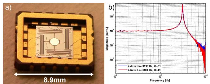
Figure 3. Gimbal-less dual-axis 4-quadrant devices used in this work: (a) typical device which reaches mechanical tilt from  $-6^\circ$  to  $+6^\circ$  on both axes. Device has a 1mm diameter mirror. (b) Small-signal characteristics of such a high-speed device
