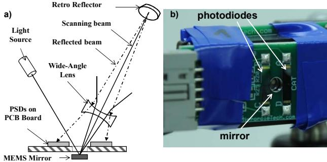
Figure 2. MEMSEye for optical 3D tracking: (a) cross-sectional schematic diagram of the methodology which eliminates the need for beam-splitters and large mirror diameters and (b) photograph of the prototype MEMSEye with a photo-sensor PCB placed in front of the scanning MEMS mirror which can be seen through a hole in the sensor PCB.
