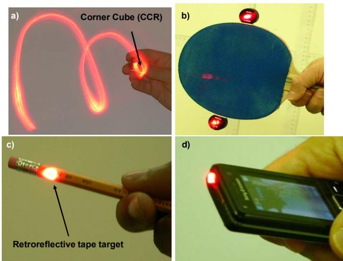
Figure 6. Examples of objects being tracked (targets are bright because the tracking system is actively pointing the laser beam onto them): (a) moving corner-cube retro-reflector, (b) a paddle-marked with two CCRs, providing orientation and position information (c) a cell-phone marked with retroreflective tape, and (d) a pencil with a retroreflective tape target.
