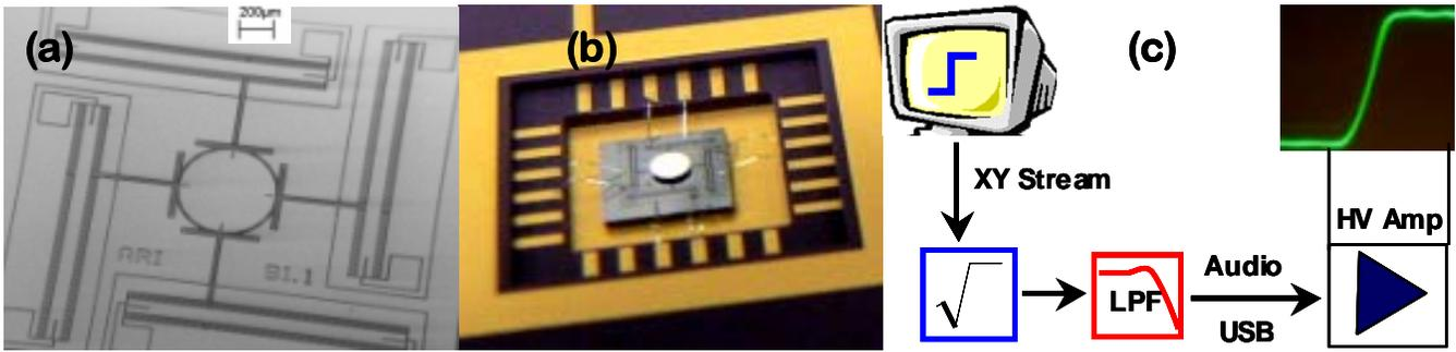
Figure 1. (a) SEM of a typical gimbal-less two-axis micromirror scanner with a monolithic 600  $\mu\text{m}$  diameter micromirror (b) device with bonded micromirror (c) Schematic of vector-display system: the desired position stream is filtered and control signals sent using audio or USB ports after stepping up the 1V output signal from the computer using a high-voltage amplifier.
